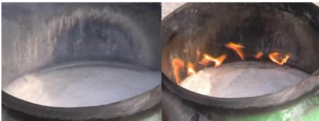
Fig 6 Tests of re-ignition effect
