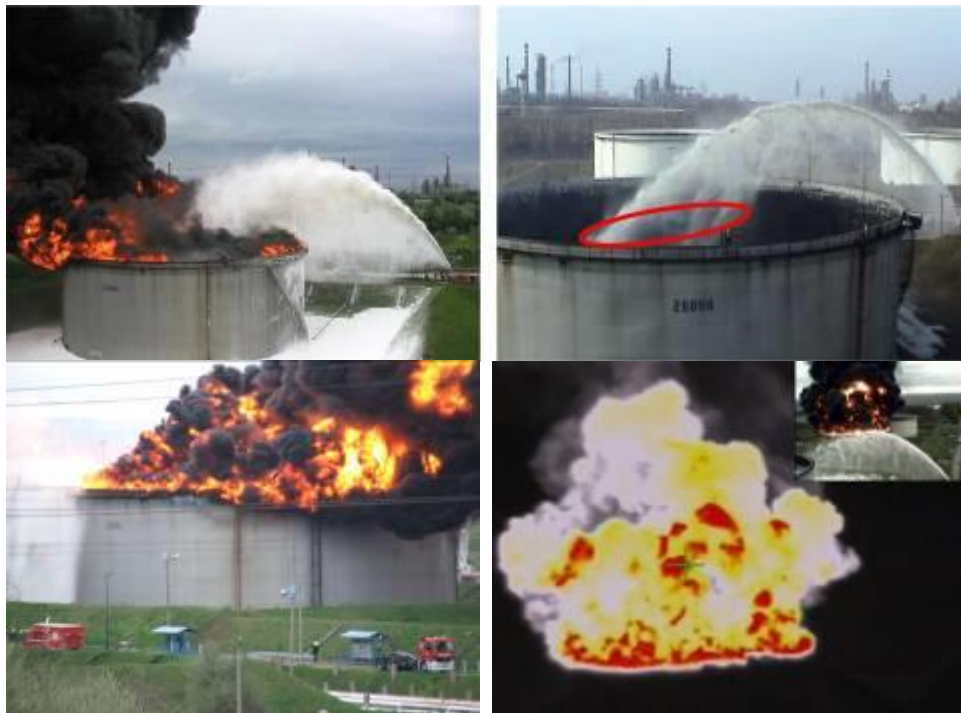
Fig 8 Firefighting test done on tank No 20.008
